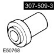
ZF Automatic transmission selector shaft seal installer 307-509-3 (LRT-44-033/3)
